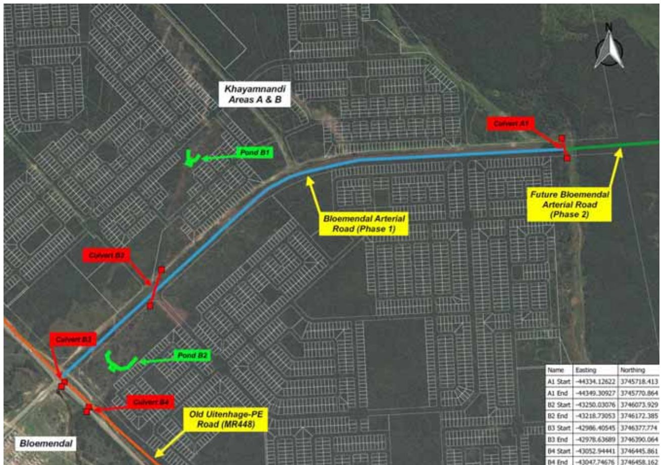
Figure 6: Culvert positions along the Bloemendal arterial.
