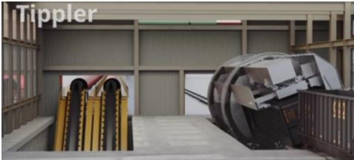
Figure 2-6: Example of the tippler
