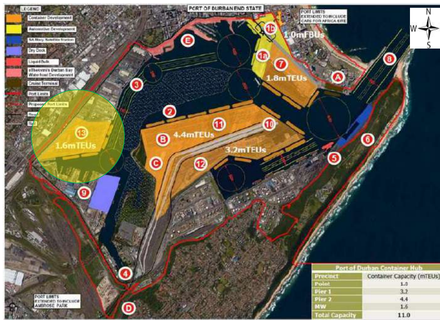
Fig.11. Port of Durban End-State, 2050, Transnet Projection. Note: Circle to Area No.13 Maydon Wharf with 'containerisation' designation.
